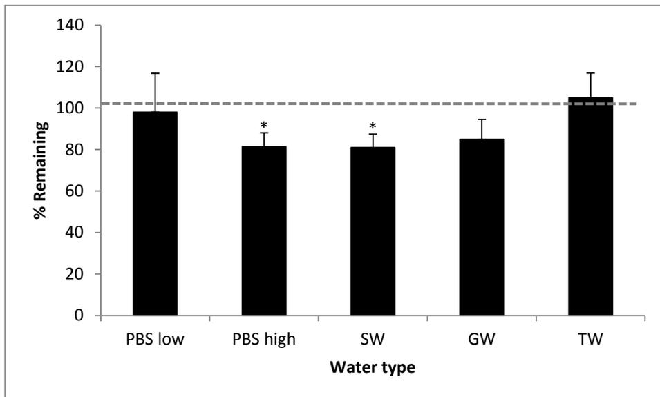
**Figure 3.3** Percent of MS2 remaining in each water type 5 hours post-spike of  $10^4$  PFU/ml into 0.1 mM PBS (PBS low), 1 mM PBS (PBS high), ground (GW), surface (SW) and dechlorinated tap water (TW) (mean; SD; n=3). Values significantly less than 100% viability are indicated with \* ( $p < 0.05$ ). Dotted line represents 100% MS2 remaining.
