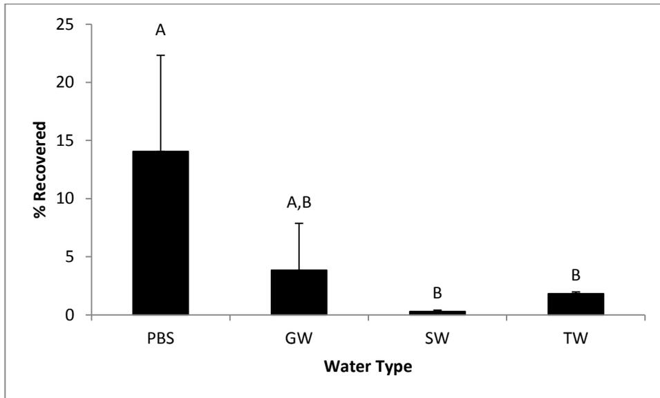
**Figure 3.2** Percent of MS2 recovered from the Zeta 60S filters post-spike of  $10^4$  PFU/ml into 10 mM PBS, ground (GW), surface (SW) and dechlorinated tap water (TW). (mean; SD; n=3)
