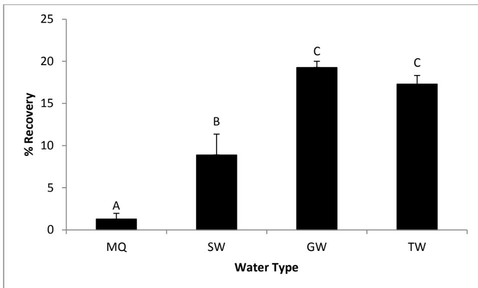
**Figure 3.5** Percent recovery of 2,4-D as determined by HPLC for MilliQ (MQ), surface water (SW), dechlorinated tap water (TW) and ground water (GW). ANOVA followed by Tukey's HSD were used to determine significant differences (A,B,C) in recovery between different water types (mean, +SD, n=3).
