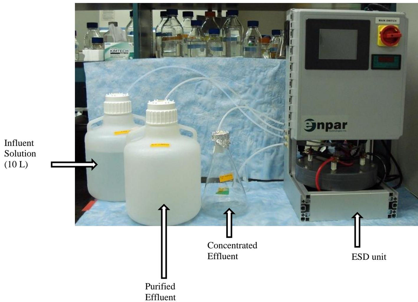
**Figure 2.1** Benchtop ESD unit and sample collection set-up.
