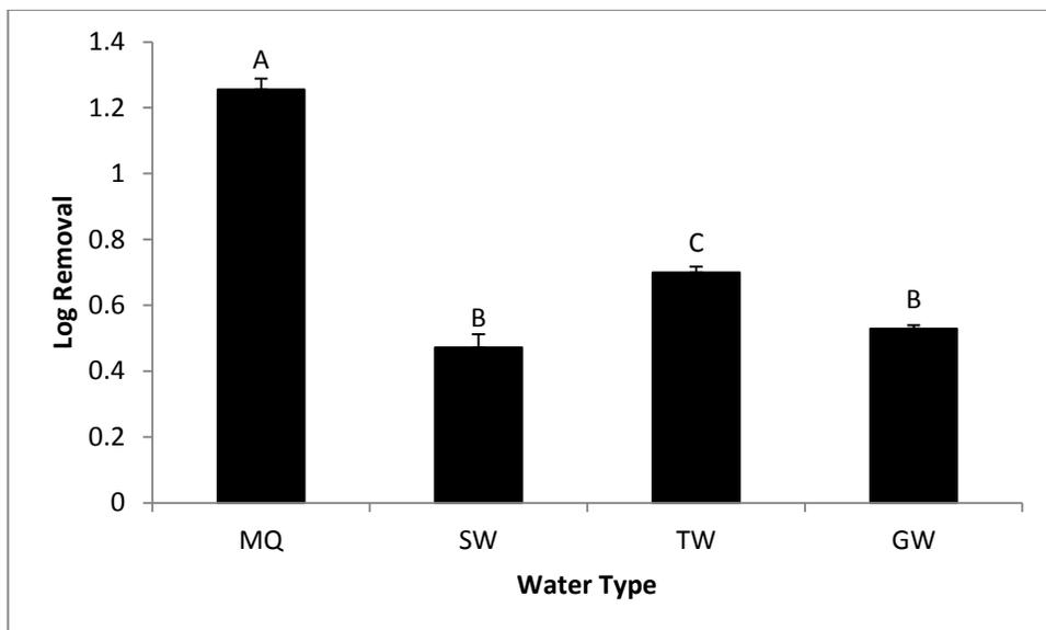
**Figure 3.4** Log removal of 2,4-D as determined by HPLC for MilliQ (MQ), surface water (SW), dechlorinated tap water (TW) and ground water (GW). ANOVA followed by Tukey's HSD were used to determine significant differences (A,B,C) in removal between different water types (mean, +SD, n=3).
