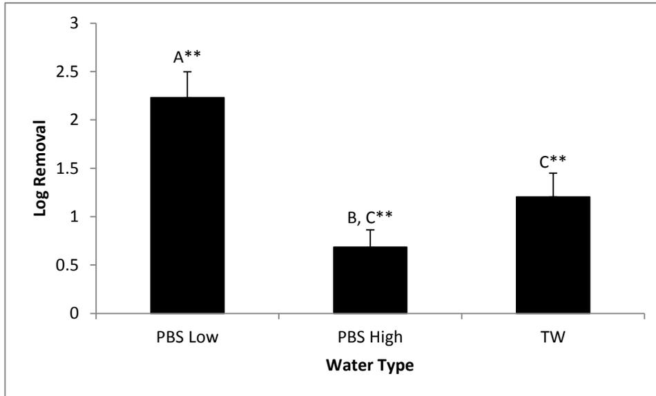
**Figure 7.1** Log removal of *E. faecalis* by CDI enumerated using A) qPCR and B) culture-based methods. ANOVA followed by Tukey's HSD were used to determine significant differences (A,B,C) within a given method for different water types, and the Student's t-test was used to determine significant differences (\*) between the two methods for a given water type (mean, +SD, n=3; \*\*p<0.01).
