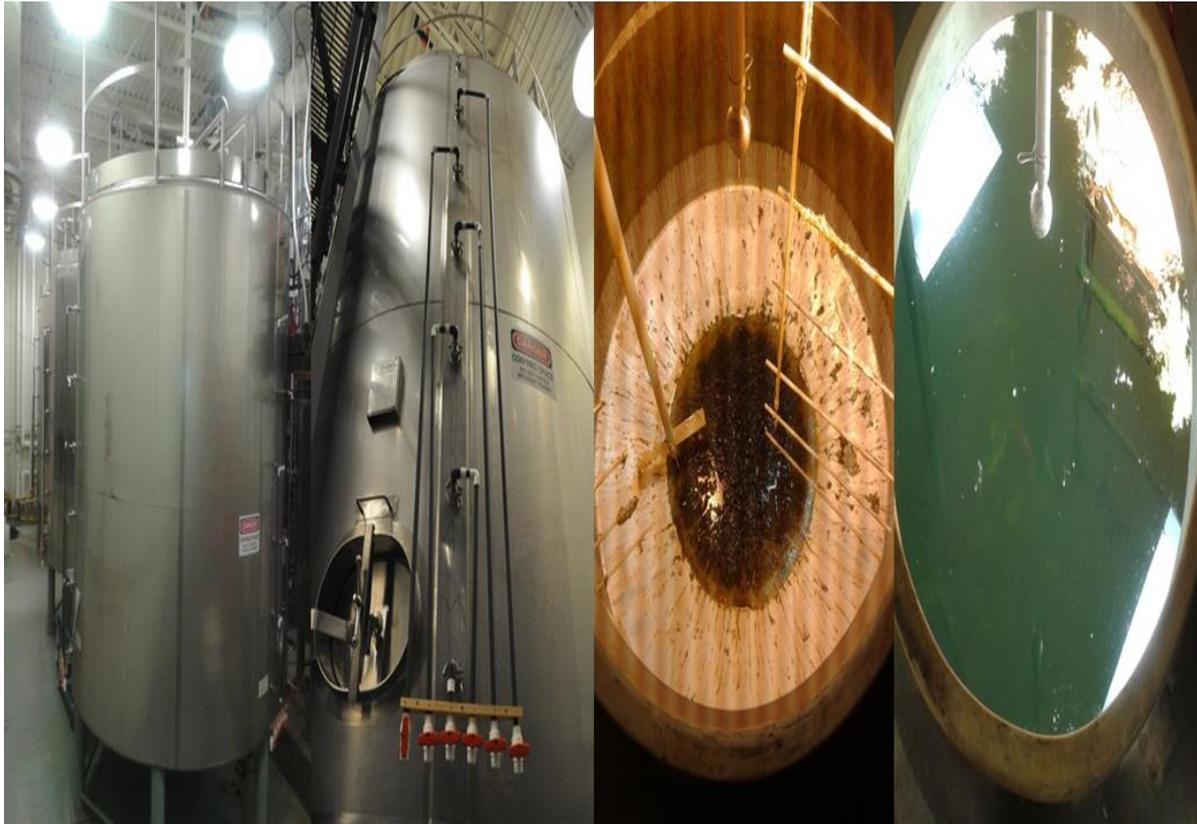
Fig. 1: From left to right: Lateral view of tanks used as mesocosms; Sampling station with six sampling ports; Overhead view of “empty” tank; Overhead view of mesocosm.
