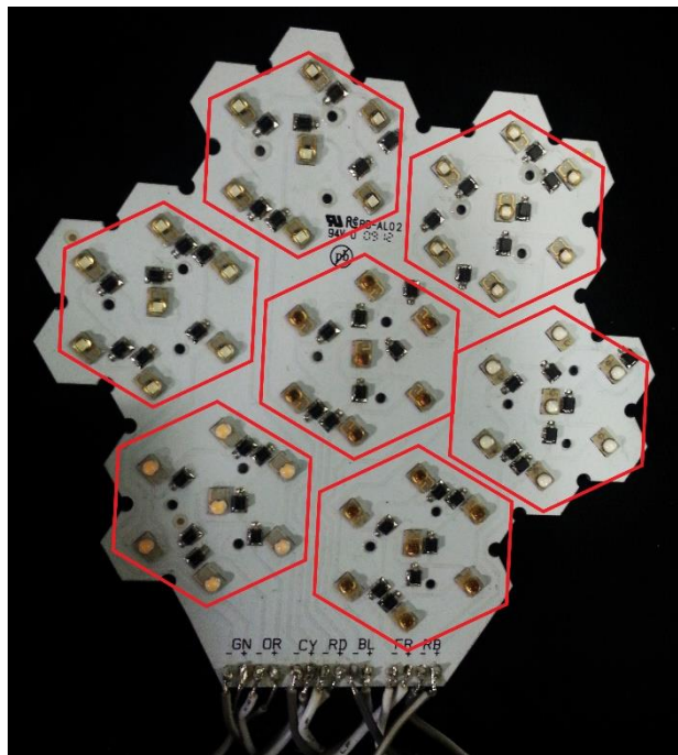
Figure 2.3: LED “star”. Each star contained seven differently coloured monochromatic LEDs on a printed circuit board (PCB). Each colour was in a cluster of seven of the same coloured LED, outlined in red. It was originally intended that each cluster of seven LEDs would have one of each of seven colours used, but the circuitry required to allow control of each colour in that scheme was unfeasible. The arrangement exercised was found to still allow for effective light mixing, despite each colour of LED being in a discrete cluster.
