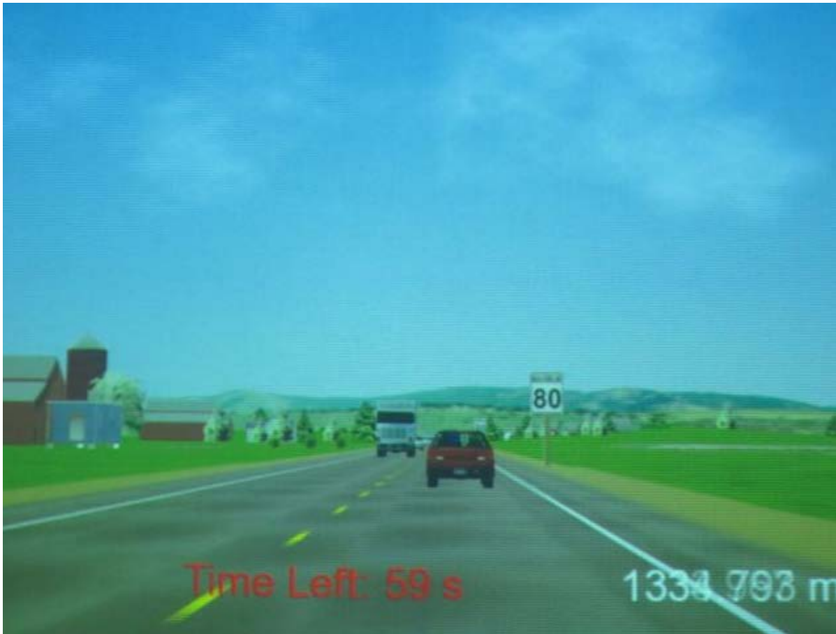
Figure 7. Screenshot of the experimental drive. The speed limit posted was 80KpH. On the left, “Time Left”, which counts down from 180 seconds, indicates how much time participants have before simulator automatically stops when the time reaches 0. On the right, the distance meter is increasing as the participant drives, and it simply refers to the distance travelled by meters.
