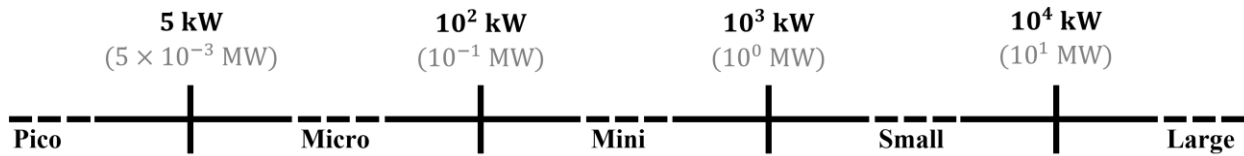
Figure 2.2: Classification of hydropower plants based on the installation capacity.
