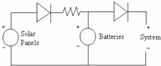
Figure 2: Logic used to regulate the power discharge from the battery.
