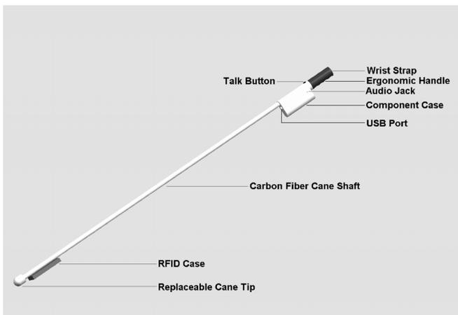
Figure 1: Detailed Cane Design
