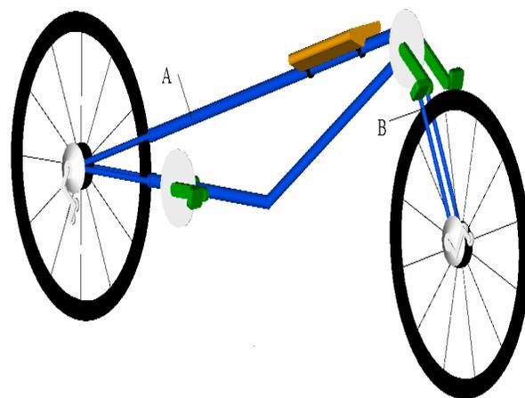
Figure 2: Prone bicycle with dual gear transmission for legs and arms
