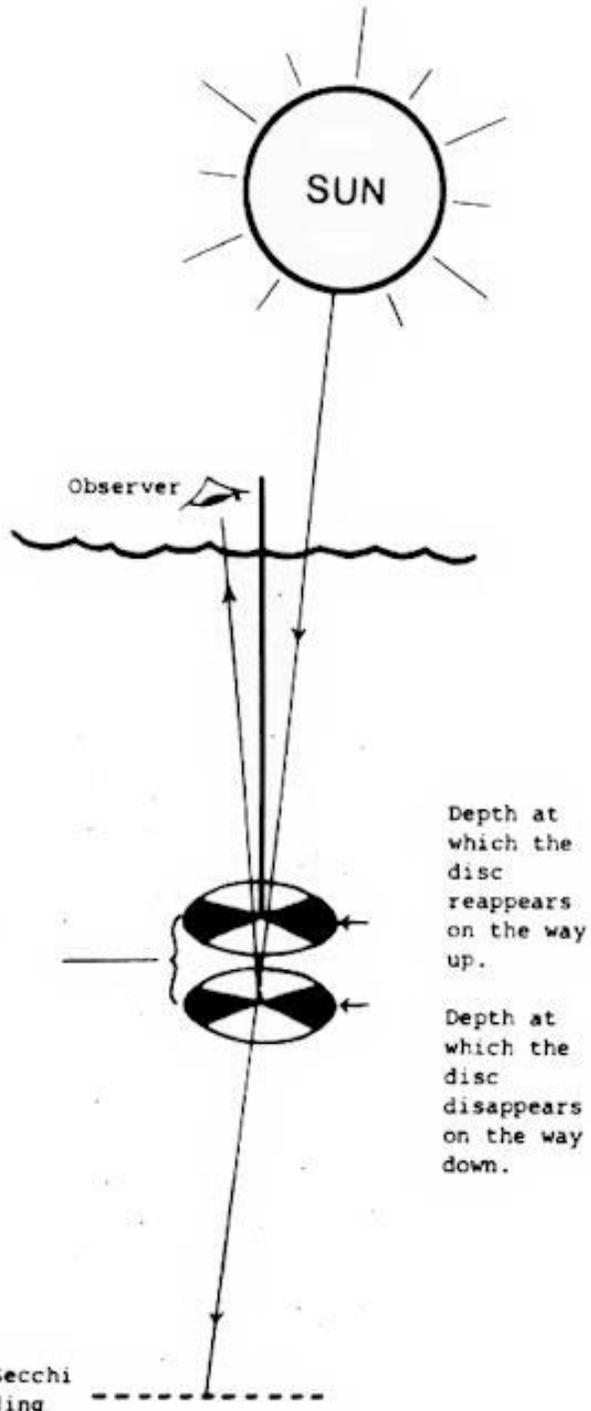
FIGURE 1: Use Of The Secchi Disc To Determine Water Clarity.
