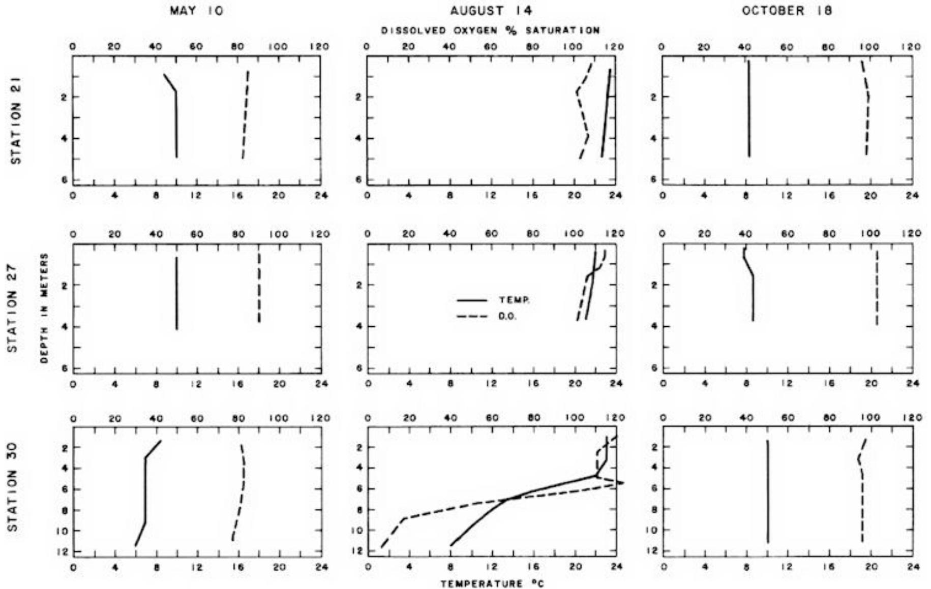
FIGURE 5: Dissolved Oxygen And Temperature Profiles.
