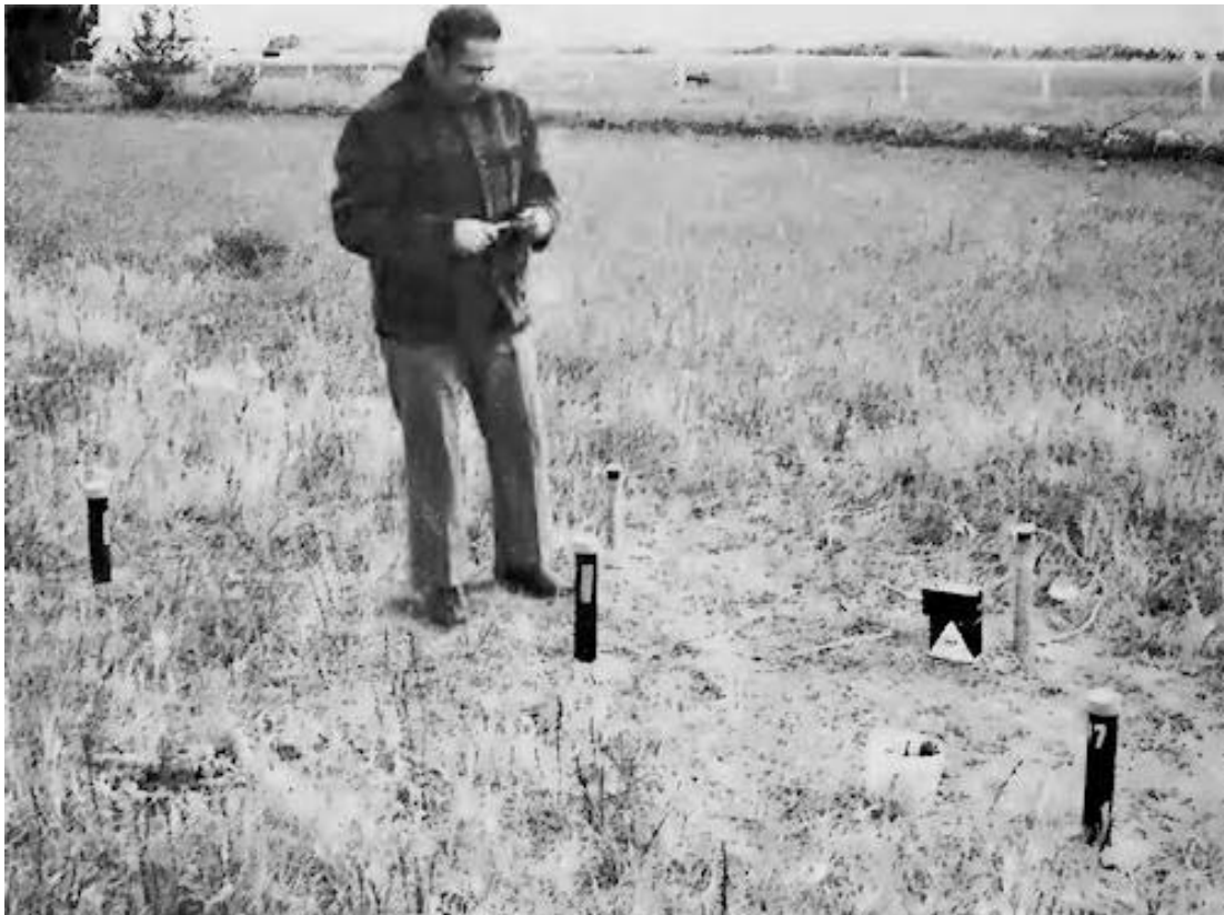
Fig. 4. A nest of piezometers used for measurement of the groundwater table at the Vegreville substation.
