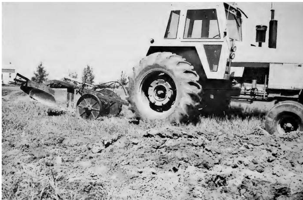
Fig. 10. Regular breaking plow that has been modified and reinforced and is capable of plowing to a 56-cm ( 22-in ) depth.
