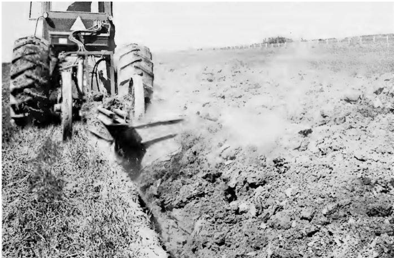
Fig. 11. Deep plowing a Solonetzic soil to a depth of 50 cm (20 in.) using a four-wheel-drive tractor.
