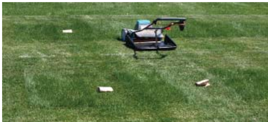
Figure 13. Clipping collection: border strips were mowed short (<40 mm) and clippings were then collected from a 0.94 m strip lengthwise in each plot using a Gardena electric reel mower set at 42 mm height of cut.
