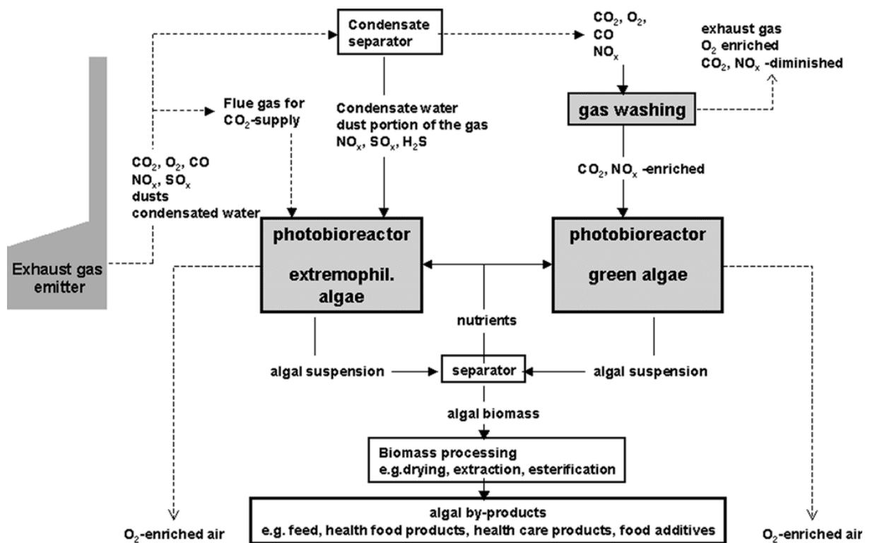
Figure 1: Scheme for CO<sub>2</sub> fixation from industrial exhaust gas by microalgae (Pulz and Gross<sup>65</sup>, reprinted from Applied Microbiology and Biotechnology (2004), vol. 65(6), pp. 635–648, with kind permission from Springer Science and Business Media, CCC licence 3623800818054)
