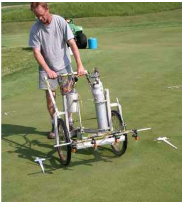
Figure 1. Application of treatments with compressed air sprayer (4 flat-fan TeeJet 8001VS nozzles at 20 psi).
