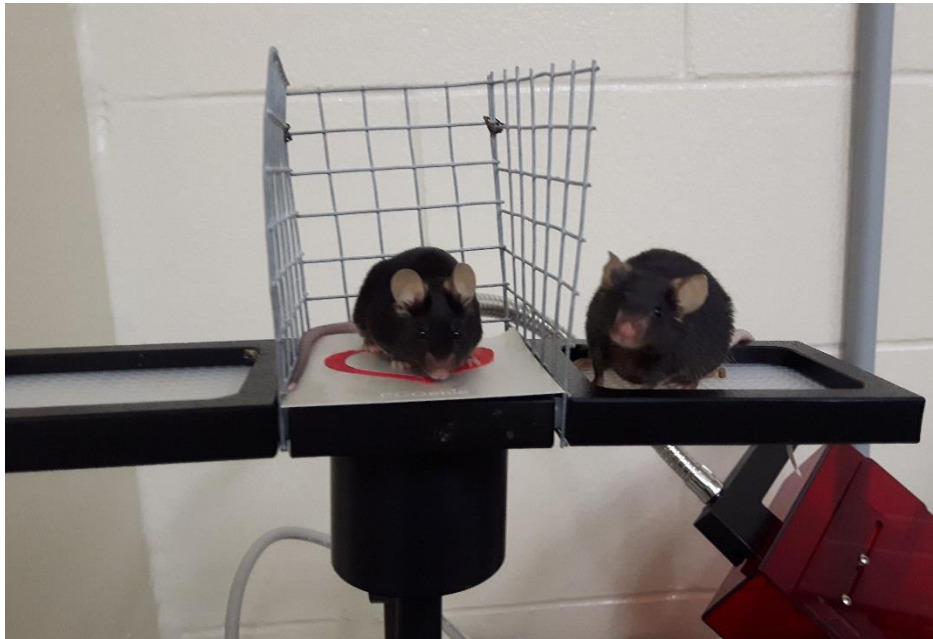
Figure AII.1 A mouse being tested on the ECGenie heart rate monitor with a cagemate on the adjacent platform. The wire mesh divider prevents the cagemate from accessing the electrode so only the focal mouse's heart rate is measured.
