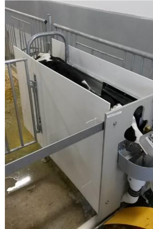
Figure 2.2: Photo of AMF with solid sides made of plastic. Photo taken at Dairy Research and Innovation Facility; Elora, Ontario.
